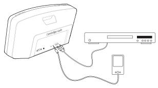
Press the MP3 or AUX button to select the analogue input and stop the playback of Bluetooth - the LED will turn to solid cyan (MP3) or solid orange (AUX).
