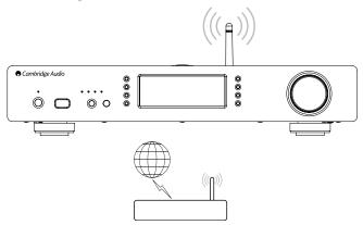
Place the Stream Magic 6 in range of your wireless network (usually 10-30m of a suitable wireless transmitter, although this is affected by walls and the construction of your building) and turn it on, via the back panel switch and then on the front panel.
