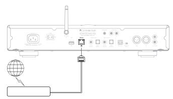
Plug one end of a network cable (Category 5/5E straight through Ethernet cable) into the LAN port on the back of the unit.
