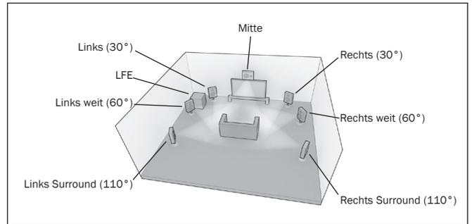
**Konfiguration 7 - 7.1-Kanal: L, C, R, LFE, Ls, Rs, Ch, Cs**
