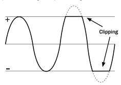
When the 651W detects clipping this LED will briefly flash. If the clipping reaches a dangerous amount that could damage the amplifier or attached speakers the unit will then go into protection.
