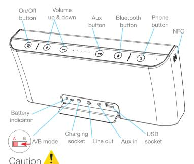
Please ensure that the mode switch is in position A for normal operation.
