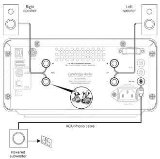
The red coloured speaker terminals are positive (+) and the black speaker terminals are negative (-). Make sure correct polarity is maintained at each speaker connector or the sound can become weak and "phasey" with little bass.
