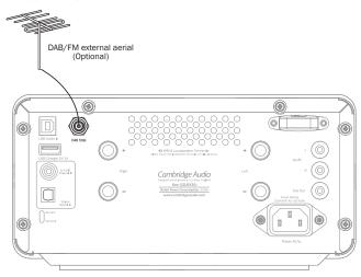
**Note:** The One is supplied with a temporary DAB/FM aerial for initial use only. For permanent use, outdoor aerials are highly recommended.
