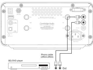
Connect to source equipment using stereo phono/RCA cables (stereo 2RCA-2RCA). Require two sets of stereo phono/ RCA cables, one for recording, one for listening.
