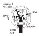
If a standard 13-amp (BS 1363) plug is used, a 3-amp fuse must be fitted or, if any other type of plug is used, a 5-amp fuse must be fitted, either in the plug or adaptor, or on the distribution board.
