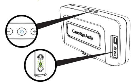
Press and hold the power button (I) on the top of the unit for one second to turn it on
