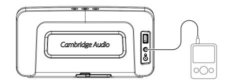
There is an Aux input on the rear of the unit that allows any analogue device to be connected. To listen to the Aux input, make sure that playback from any paired Bluetooth device is paused. When no Bluetooth audio is playing, your Minx Go will automatically play the Aux input.
