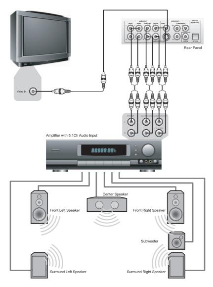
The built-in Dolby Digital decoder inside your 50-series DVD player makes it possible to play discs recorded with Dolby Digital. This is achieved simply by connecting your player to an amplifier or receiver with 5.1 channel amplification and an appropriate home theatre loudspeaker package.
