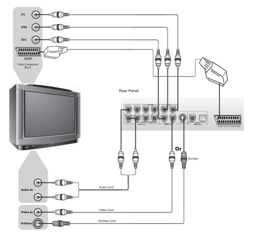
If your TV has S-Video inputs, an S-Video interconnect can be used to connect this player. When the video output is used the component video outputs cannot be used.
