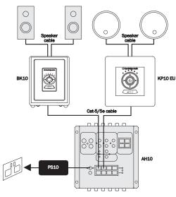
Note: When using a BK10 keypad with an AH10 hub, an Incognito PS10 power supply unit MUST be used.
