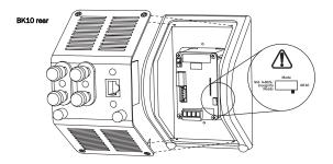
Note: Setting the mode switch to the wrong setting can cause erroneous operation!
