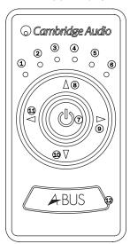
① - ⑥ The six LEDs indicate the volume level of the BK10. The LEDs also also display the source selected when the source is changed and can also show the status of some other functions. For full instructions on volume adjustment, source selection, sound adjustment and local source selection modes, refer to the 'Operating instructions' section of this guide.
