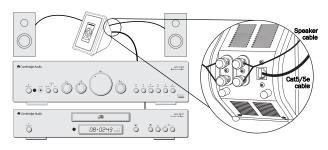
The BK10 comes with 10 metres of Cat5 connection cable, but an Incognito CP20 cable pack (with 20 metres of cable, 2 x 3.5-3.5 connection cables and a punch-down/wire stripper tool) can be purchased separately.
