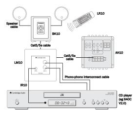
The local source selection mode will need to be activated to configure the BK10 correctly. This mode is only available when the Mode Switch is set to "AH10" mode. LM10s can only be used with an AH10 hub.
