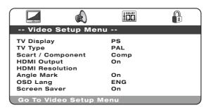
With the Video Setup menu selected, use the ▲ and ▼ arrows to move up/down to the desired sub-menu. Use the navigation arrows (▲ ▼ ◀ ▶ ) to adjust the settings and press the *Enter* button to confirm your selection. The following list shows the Video Setup menu structure:
