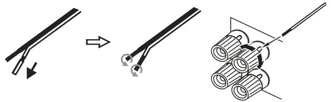
**Note:** All connections are made via loudspeaker cable, except if using an active subwoofer which would be connected via a standard RCA phono cable. Banana Plugs (4mm standard) connected to the speaker cable are recommended for direct insertion into the speaker terminals.
