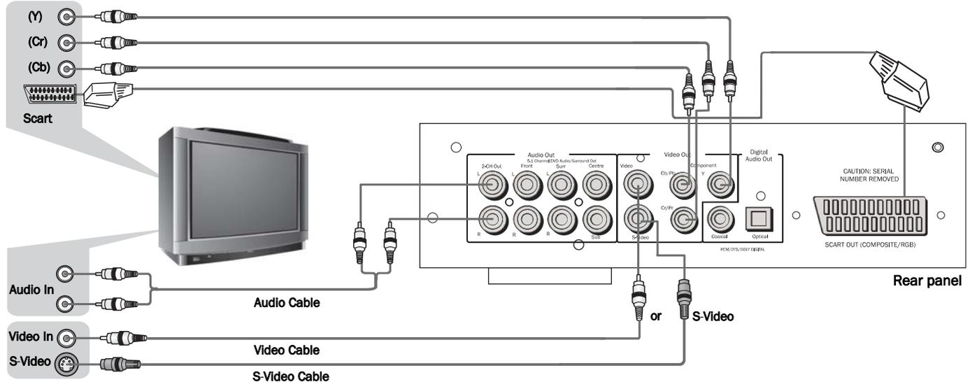
If your TV has S-Video inputs, an S-Video interconnect can be used to connect this player. When the S-Video output is used the component video outputs cannot be used.
