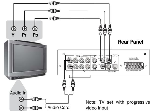
If your progressive scan TV has Y, Pb Pr video inputs you can use the players Y, Cb/Pb, Cr/Pr outputs . Press the p-Scan button to switch the player to the progressive scan video output mode.
