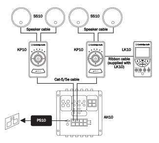
Important: LK10 will only operate when connected to KP10 as part of a complete AH10 hub-based system. It is not compatible with 'Incognito Ready' amplifiers.
