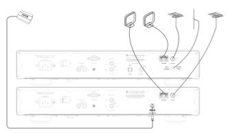
**Note:** The 650T is supplied with temporary FM or DAB aerials for initial use only. For permanent use, outdoor aerials are highly recommended.
